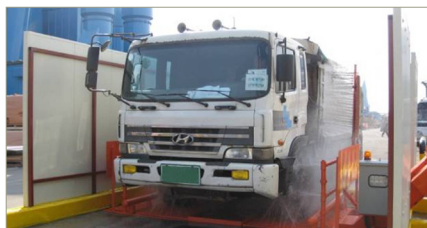
Wheel-cleaning facilities the Incheon Plant
