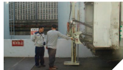
Inspection of soil contamination around oil tanks
