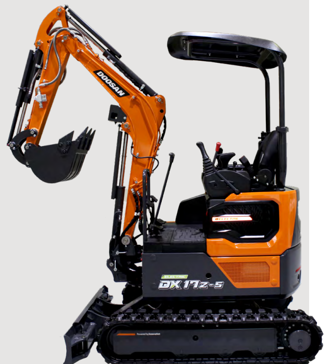
Prototype of 1.7-ton electric excavators (DX17ZE)
